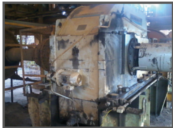
Original gearbox SF 1.52 (Cap. 1219hp), Weight: 5765kg Triple Reduction, Motor Pump without fan
