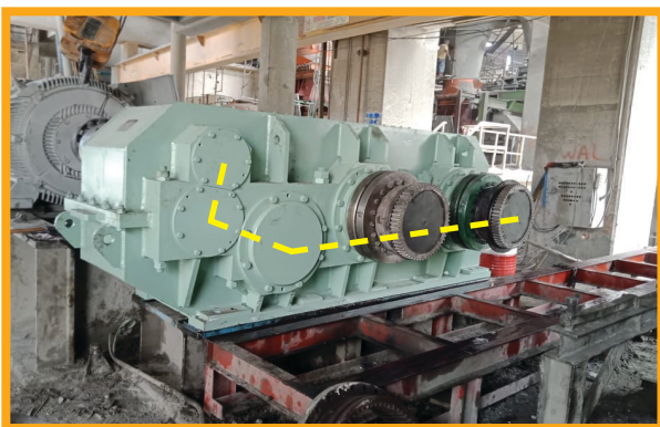
Drop-in gearbox with oversized gears and pinions (offset gear arrangement) that followed existing dimensions of mounting and shaft. Significant increase in gearbox mechanical rating
