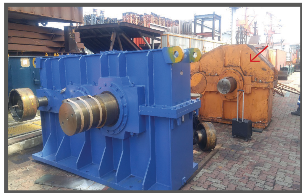
Original obsolete main hoist Gearbox (in Orange)
