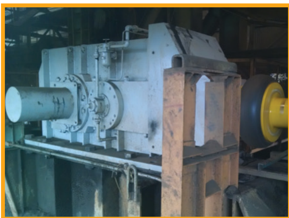
Drop-in gearbox SF 2.24 (Cap. 1792hp), Weight: 4859kg Double Reduction, Shaft Pump with one cooling fan
