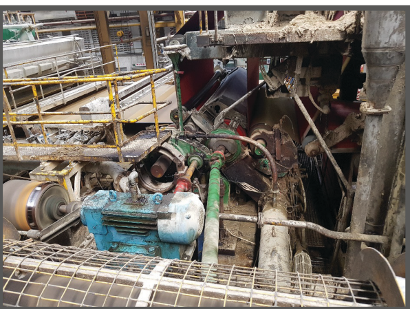
Original Worm Gear overheated and was prone to oil leaks causing issues for maintenance.
