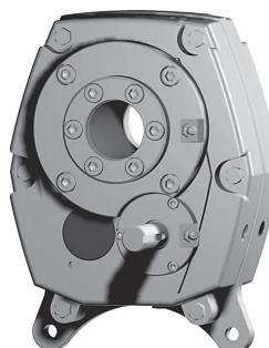
The HSM can be secured to the driven shaft by means of the Taper-Grip® bush which will transmit the torque and shock overload capacity of the selected gearbox.
