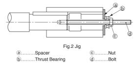
The hollow shaft is made according to the tolerances of JIS H8. If you experience impact or notice a large radial load with the hollow shaft, further tighten the fitting between the hollow shaft and the driven shaft. (We recommend JIS js6 or k6 as the tolerance of a driven shaft.)
