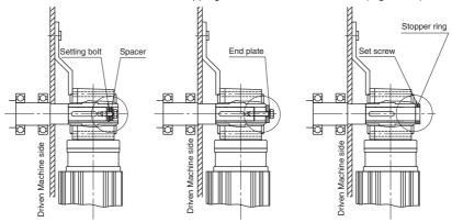
Fig.13 Fixed by stopping shaft
