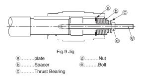
The hollow shaft is made according to the tolerances of JIS H8. If you experience impact or notice a large radial load with the hollow shaft, further tighten the fitting between the hollow shaft and the driven shaft, (We recommend JIS js6 or k6 as the tolerance of a driven shaft.)
