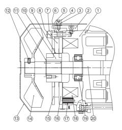
2 Release fitting 3 Stud bolt 4 Adjusting washer 5 Manual release prevention spacer 6 Brake release bolt 7 Spring washer 8 Gap adjusting nut 9 Brake lining 10 Boss Shaft retaining C-ring 11 Cover 12 13 Spring pin 14 Fan 15 Leaf spring 16 Fixed plate 17 Armature core 18 Spring Electromagnetic coil 19 20 Ball bearing 21 Motor shaft
