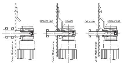
Fig.10 Fixed by spacer and plate
