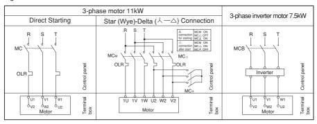
MC: Electromagnetic contactor
