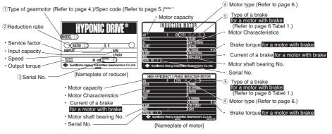
Fig. 1-b Nameplate of Gearmotor (Type II)
