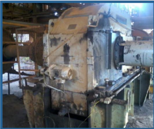
Original gearbox SF 1.52 (Cap. 1219hp), Weight: 5765kg
