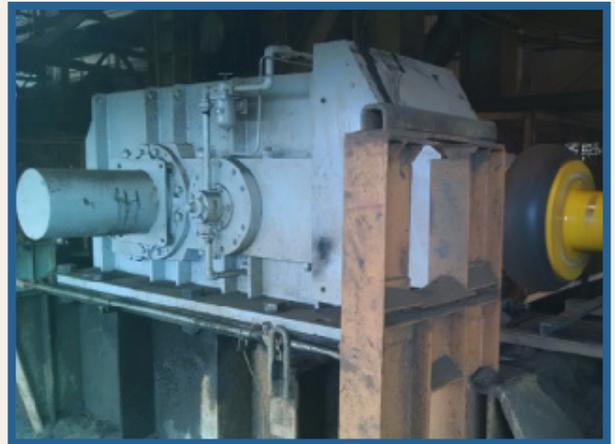
Drop-in gearbox SF 2.24 (Cap. 1792hp), Weight: 4859kg
