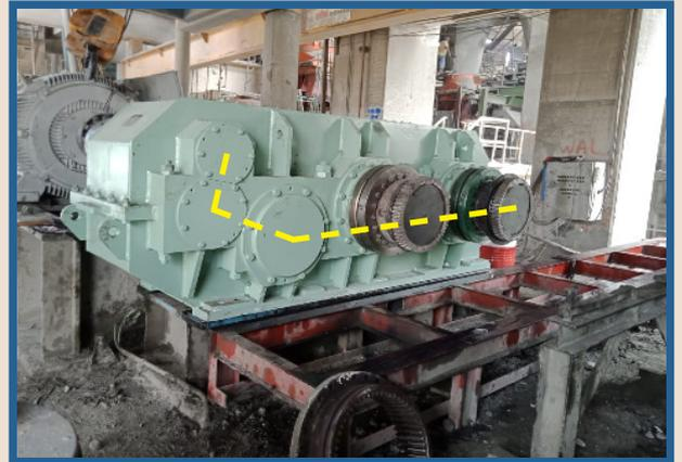
Drop-in gearbox with oversized gears and pinions (offset gear arrangement) that followed existing dimensions of mounting and shaft. Significant increase in gearbox mechanical rating.
