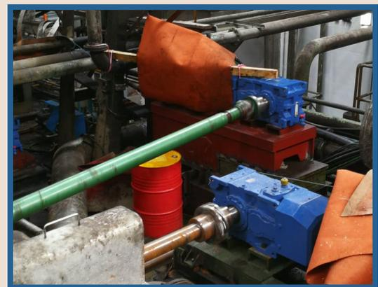
Replacement of our Paramax Right Angle, equipped with Double Reduction with fan, <60C max operating temperature with new baseplate.
